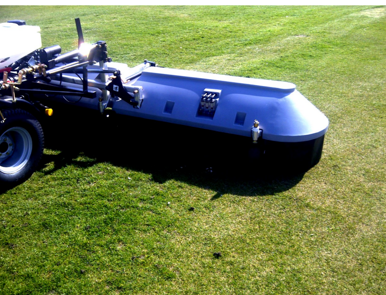
One complete tunnel across the whole boom with no gaps for wind to alter the spray pattern
