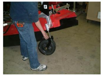
Figure 3: Inserting castor wheel
