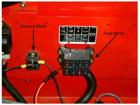
Figure 25: Power wire connections under drives seat
