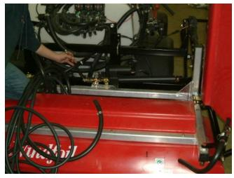
Figure 17: Wing Actuator Adjustment
