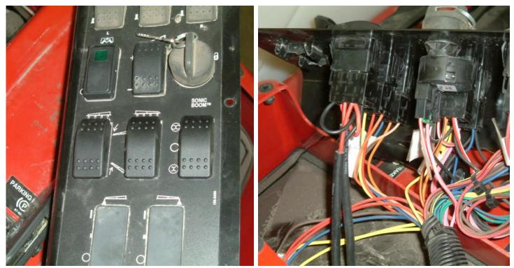
Figure 21: Rocker Switches in Console Panel
