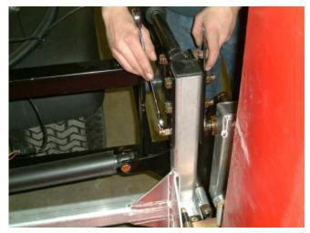
Figure 18: Wing stop adjustment
