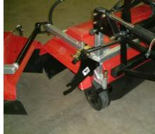
Figure 14: Extend wing actuator
