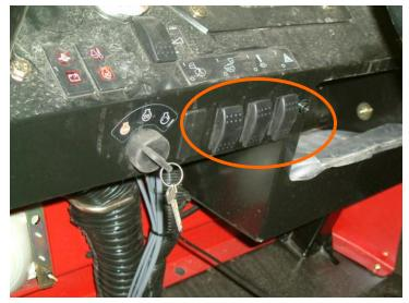
Figure 23: Dash of 5800 with inserted switches
