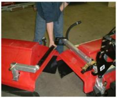
Figure 13: Attaching break away tube to center section
