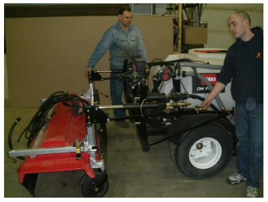
Figure 8: Positioning center section around boom mount assembly
