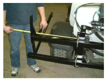
Figure 2: Boom mount assembly
