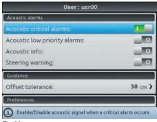
It allows to enable/disable the acoustic signal when new Critical alarms are triggered (Fig. 97).
