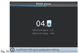
"PDOP" is the parameter that depends on the position and number of satellites in space that affect the positional precision of the system (longitude and latitude); the lower the value, the higher is the driving precision.
