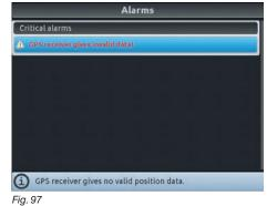
Navigator features an **Alarm** menu (Fig. 97, accessible from the "Home" menu by pressing F6). This page displays all active notifications for the operator.
