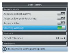
It allows to enable/disable the acoustic signal when the operator must steer in order to align the machine with the following track, avoiding unsprayed or overlapping areas between the two sprays (**Steering** radius set in par. 10.1.2 Working parameters).
