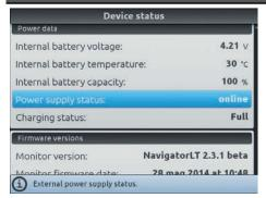
The device checks the status of the power supply.
