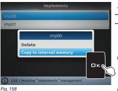
Allows to copy data from the pendrive onto Navigator internal memory.
