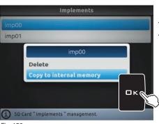
Allows to copy data from the SD card onto Navigator internal memory.
