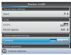
Navigator can connect to up to 2 cameras in order to monitor the working areas that the operator is unable to see (e.g., when driving in reverse).
