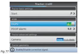
Allows to enable / disable the DGPS (SBAS) differential correction function
