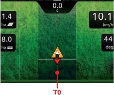
When this function is used, Navigator deletes the previous reference track TO (if present), and prompts the operator to save two NEW points A and B on the field, which create a NEW reference track.
