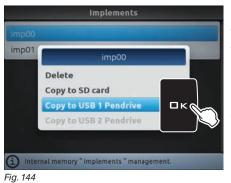
Allows to copy data from Navigator internal memory onto a pendrive.
