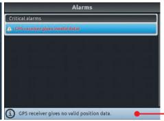
A description of the selected notification is shown at the bottom of the display.
