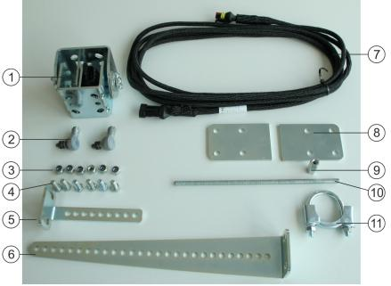
Wheel angle sensor: Components for installation
