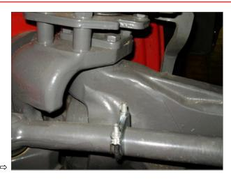
**6.** Screw the adapter plate onto the casing of the wheel angle sensor. Select the large or small plate.
