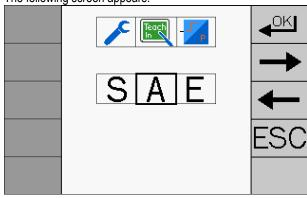
4. Mark the "A" icon when the pressure sensor supplies a current signal. This is how a pressure sensor mounted by default works. Set "E" when the pressure sensor supplies a voltage signal. Set "S" when it is a flow switch.
